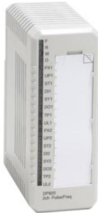
DP820 is a two-channel pulse counting module for incremental pulse transmitters up to 1.5 MHz. Each channel contains counters and registers for position/length and speed/frequency measurement. Each channel provides three balanced inputs for connection of a pulse transmitter, one digital input and one digital output. Pulse transmitters with RS422, +5 V, +12 V, +24 V and 13 mA interfaces can be connected to DP820.
