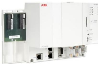
This CPU module is the lite base unit of the Freelance AC 900F controller family. It typically supports up to 400 I/Os and 3 MB battery-buffered SRAM. 3 Ethernet interfaces, 400 MHz CPU clock, 11 MB Controller Memory, 3 MB battery buffered SRAM, 8 MB DRAM. 2 slots for assembling Communication Interface Modules.
