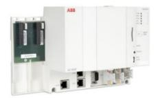
This CPU module is the lite base unit of the Freelance AC 900F controller family. It typically supports up to 400 I/Os and 3 MB battery-buffered SRAM. 3 Ethernet interfaces, 400 MHz CPU clock, 11 MB Controller Memory, 3 MB battery buffered SRAM, 8 MB DRAM. 2 slots for assembling Communication Interface Modules.
