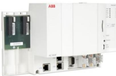
This CPU module is the lite base unit of the Freelance AC 900F controller family. It typically supports up to 400 I/Os and 3 MB battery-buffered SRAM. 3 Ethernet interfaces, 400 MHz CPU clock, 11 MB Controller Memory, 3 MB battery buffered SRAM, 8 MB DRAM. 2 slots for assembling Communication Interface Modules.
