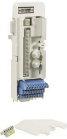
The TU891 is a compact MTU for the S800 I/O. The MTU is a passive unit used for connection of the field wiring and power supply to the I/O modules. It also contains a part of the ModuleBus. The TU891 MTU has gray terminals for field signals and process voltage connections. The maximum rated voltage is 50 V and maximum rated current is 2 A per channel, but these are primarily constrained to specific values by the design of the I/O modules for their certified application.
