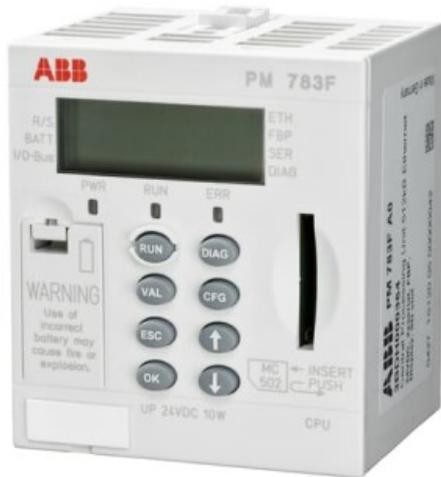
This is the smallest Freelance CPU that typically supports up to 300 I/Os. It optionally can be equipped with 8 direct I/O modules and one Profibus Interface module and supports Modbus TCP. Two serial line interfaces complement the connectivity. One interface can be used for Modbus communication, while the other is used for diagnosis.
