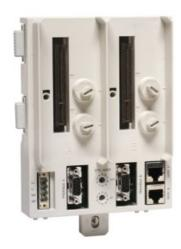
The TU846 is a module termination unit (MTU) for redundant configuration of the field communication interface CI840/CI840A and redundant I/O. The MTU is a passive unit having connections for power supply, two electrical ModuleBuses, two CI840/CI840A and two rotary switches for station address (0 to 99) settings.
