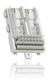
The TU844 MTU can have up to 8 I/O channels and 2+2 process voltage connections. Each channel has two I/O connections and one ZP connection. Input signals are connected via individual shunt sticks, TY801. The shunt stick is used to choose between voltage and current input. The maximum rated voltage is 50 V and maximum rated current is 2 A per channel.
