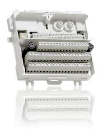
The TU830V1 MTU can have up to 16 I/O channels and two process voltage connections. Each channel has two I/O connections and one ZP connection. The MTU is a passive unit used for connection of the field wiring to the I/O modules. It also contains a part of the ModuleBus.
