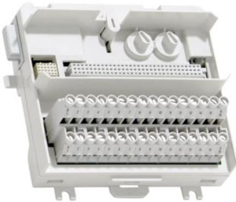
The TU851 MTU can have up to 16 I/O channels. The maximum rated voltage is 250 V and maximum rated current is 3 A per channel. The MTU distributes the ModuleBus to the I/O module and to the next MTU. It also generates the correct address to the I/O module by shifting the outgoing position signals to the next MTU.
