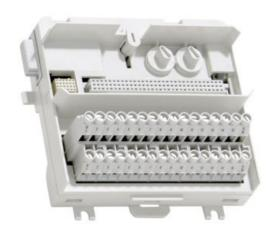
The TU851 MTU can have up to 16 I/O channels. The maximum rated voltage is 250 V and maximum rated current is 3 A per channel. The MTU distributes the ModuleBus to the I/O module and to the next MTU. It also generates the correct address to the I/O module by shifting the outgoing position signals to the next MTU.
