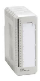
This module has 16 digital outputs. The maximum continuous output current per channel is 0.5 A. The outputs are current limited and protected against over temperature. The outputs are divided into two groups with eight output channels and one voltage supervision input in each group. Each output channel consists of a current limited and over temperature protected high side driver, EMC protection components, inductive load suppression, output state indication LED and optical isolation barrier.
