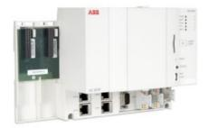
This CPU module is the medium base unit of the Freelance AC 900F controller family. It typically supports up to 1500 I/O and 8 MB battery buffered SRAM. 4 Ethernet interfaces, 800 MHz CPU clock, 24 MB Controller Memory, 8 MB battery buffered SRAM, and 16 MB DRAM. 2 slots for assembling Communication Interface Modules.
