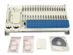
The remote S900 I/O system can be installed in non-hazardous areas or directly in Zone 1 or Zone 2 hazardous area depending on the selected system variant. S900 I/O communicates with the control system level using the PROFIBUS DP standard. The I/O system can be installed directly in the field, therefore the costs for marshalling and wiring are reduced.
