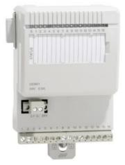
The DO801 is a 16 channel 24 V digital output module for the S800 I/O. The output voltage range is 10 to 30 volt and the maximum continuous output current is 0.5 A. The outputs are protected against short circuits, over voltage and over temperature. The outputs are in one isolated group. Each output channel consists of a short circuit and over temperature protected high side driver, EMC protection components, inductive load suppression, output state indication LED and optical isolation barrier.
