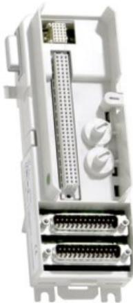
The TU819 is a 50 V compact module termination unit (MTU) for the S800 I/O system with 32 signal connections. The MTU is a passive unit used for connection of the field wiring. It also contains a part of the ModuleBus.
