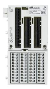
The I/O Terminal Units TU 715F (screw type terminal) and TU 716F (spring type terminal) are used as a socket for the I/O module, which exclusively incorporates inputs and outputs for 24V DC digital or analog signals.
