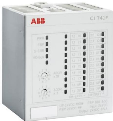
A PROFIBUS Slave communication interface for use with S700 I/O. It has also 8 digital inputs, 8 digital outputs, four analog inputs, and two analog outputs. 1 x Interface (Sub-D plug) for PROFIBUS DP 8 DI: 24 V DC 8 DO: 24 V DC/0.5 A 4 AI: +10 V, 0/4-20 mA, 24 V DC, RTD 2 AO: +10 V, 0/4-20 mA, 24 V DC 12 Bit + sign, 2-wire, 24 V DC 5 W 1-wire, 24 V DC 100 W Use with TU 709F / TU 710F
