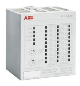
A PROFIBUS Slave communication interface for use with S700 I/O. It has also 8 digital inputs, 8 digital outputs, four analog inputs, and two analog outputs. 1 x Interface (Sub-D plug) for PROFIBUS DP 8 DI: 24 V DC 8 DO: 24 V DC/0.5 A 4 AI: +-10 V, 0/4-20 mA, 24 V DC, RTD 2 AO: +-10 V, 0/4-20 mA, 24 V DC 12 Bit + sign, 2-wire, 24 V DC 5 W 1-wire, 24 V DC 100 W Use with TU 709F / TU 710F
