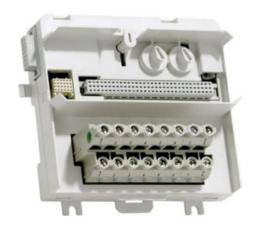
The TU831V1 MTU can have up to 8 I/O channels. The maximum rated voltage is 250 V and maximum rated current is 3 A per channel.
