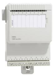
The DI802 is an 8 channel 120 V a.c./d.c. digital input module for the S800 I/O. This module has 8 digital inputs. The a.c. input voltage range is 77 - 130 volt and the input current is 10 mA at 120 V a.c. The d.c. input range is 75 - 145 V and the input current is 2.8 mA at 110 V. The inputs are individually isolated. Every input channel consists of current limiting components, EMC protection components, input state indication LED and optical isolation barrier.
