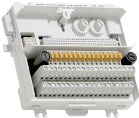
The TU850 MTU can have up to 16 I/O channels. The maximum rated voltage is 50 V and maximum rated current is 15mA per I/O channel (digital input) or 25mA per two I/O channels (analog input).
