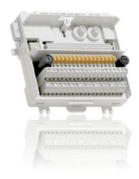
The TU850 MTU can have up to 16 I/O channels. The maximum rated voltage is 50 V and maximum rated current is 15mA per I/O channel (digital input) or 25mA per two I/O channels (analog input).
