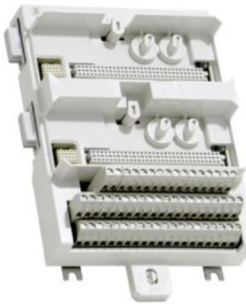
The TU843 MTU can have up to 16 I/O channels and 2+2 process voltage connections. Each channel has two I/O connections and one ZP connection. The maximum rated voltage is 50 V and maximum rated current is 3 A per channel.
