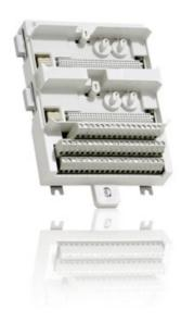
The TU843 MTU can have up to 16 I/O channels and 2+2 process voltage connections. Each channel has two I/O connections and one ZP connection. The maximum rated voltage is 50 V and maximum rated current is 3 A per channel.
