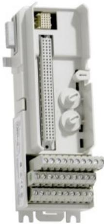
The TU810/TU810V1 is a 16 channel 50 V compact module termination unit (MTU) for the S800 I/O. The MTU is a passive unit used for connection of the field wiring to the I/O modules. It also contains a part of the ModuleBus.
