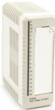
The DO828 is an 16 channel 125V d.c. / 250V a.c. relay output module for the S800 I/O. The maximum output voltage is 125V d.c. / 250V a.c. and the maximum continuous output current is 2A. All outputs are individually isolated.
