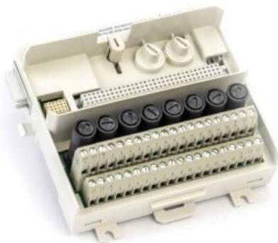
The TU838 MTU can have up to 16 I/O channels. The maximum rated voltage is 50 V and maximum rated current is 3 A per channel.
