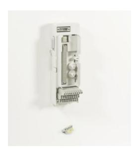
The TU891 MTU has gray terminals for field signals and process voltage connections. The maximum rated voltage is 50 V and maximum rated current is 2 A per channel, but these are primarily constrained to specific values by the design of the I/O modules for their certified application. The MTU distributes the ModuleBus to the I/O module and to the next MTU. It also generates the correct address to the I/O module by shifting the outgoing position signals to the next MTU.
