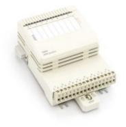
The DI803 is an 8 channel 230 V a.c./d.c. digital input module for the S800 I/O. This module has 8 digital inputs. The a.c. input voltage range is 164 - 264 volt and the input current is 7.6 mA at 230 V a.c. The d.c. input range is 175 - 275 V and the input current is 1.6 mA at 220 V. The inputs are individually isolated. Every input channel consists of current limiting components, EMC protection components, input state indication LED and optical isolation barrier.
