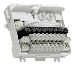
The TU837V1 MTU can have up to 8 I/O channels. The maximum rated voltage is 250 V and maximum rated current is 3 A per channel. The MTU distributes the ModuleBus to the I/O module and to the next MTU. It also generates the correct address to the I/O module by shifting the outgoing position signals to the next MTU.
