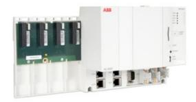
This CPU module is the high-end base unit of the Freelance AC 900F controller family. It typically supports up to 1500 I/Os. 4 Ethernet interfaces, 800 MHz CPU clock, 48 MB Controller Memory: 16 MB battery buffered SRAM, 32 MB DRAM. 4 slots for assembling Communication Interface Module.
